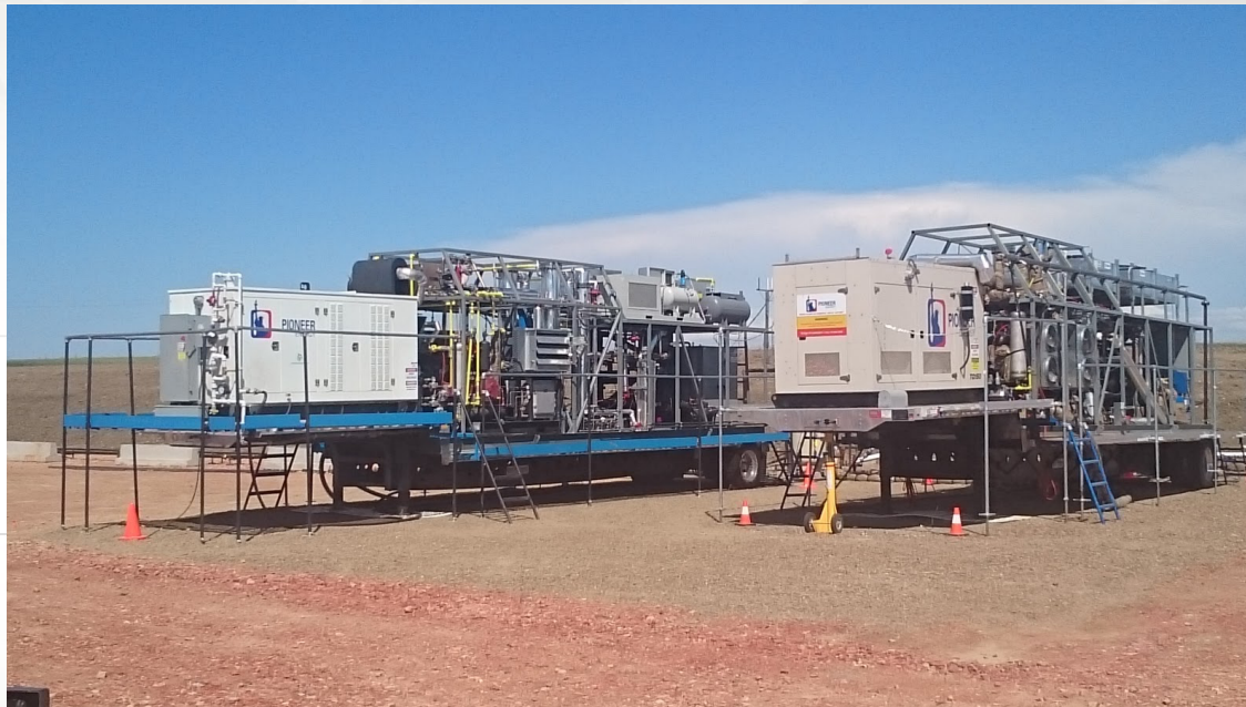
Pioneer Flare gas capture machines, 2 Flarecatcher™ deployed to Bakken flare site, North Dakota, 2015.
